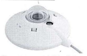
05 pyranometers to measure solar irradiation and data logger to record digital data
