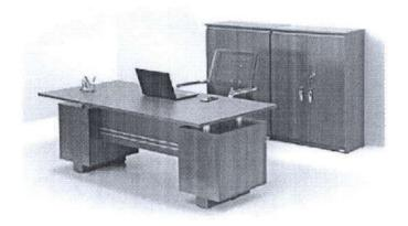
Top, modesty panel and side panels should be minimum 22mm thickness particle board, double-sided HPM and 2mm thick ABS edge finish. Modesty panel maximum height Approx. 375mm. Top and side panel are met in 45 cutting type. Finishing colour to be decided from manufacturer standard ranges.
