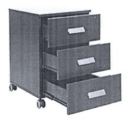
Side table with 3 drawers equally sized. Top, and side panels should be minimum 22mm thickness particle board, double-sided HPM and 2mm thick ABS edge finish. All fixing details shall be covered in closed position.
