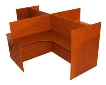
Top, modesty panel and side panels should be minimum 22mm thickness particle board, double-sided HPM and 2mm thick ABS edge finish. Modesty Panel maximum height approx. 375mm. Top and side panel are met in 45 cutting type. Finishing colour to be decided from manufacturer standard ranges.
