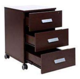
Side table with 3 drawers equally sized. Top, and side panels should be minimum 22mm thickness particle board, double-sided HPM and 2mm thick ABS edge finish. All fixing details shall be covered in closed position.
