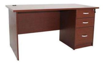
Top, modesty panel and side panels should be minimum 22mm thickness particle board, double-sided HPM and 2mm thick ABS edge finish. Modesty panel maximum height approx. 375mm. Top and side panel are met in 45 cutting type. Finishing colour to be decided from manufacturer standard ranges.
